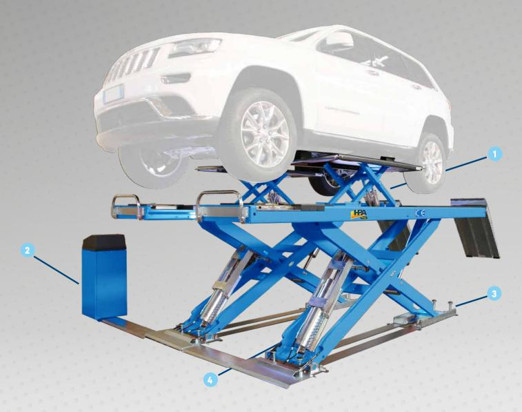
1. Lift table with double lifting cylinder to ensure a constant parallel lift movement.
