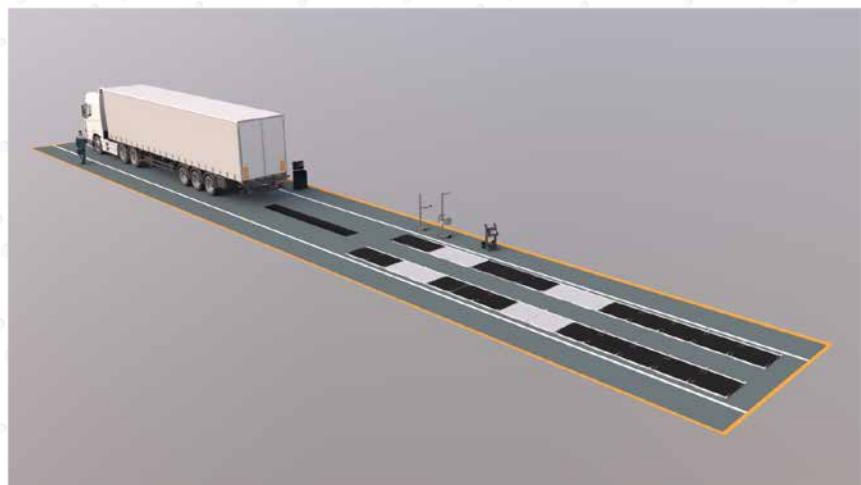
*With this configuration, the tractor and the trailer of the vehicle under test are tested through a single braking.*
