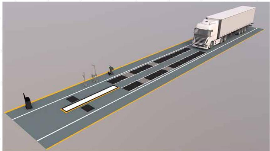
*With this configuration, the tractor and the trailer of the vehicle under test are tested through a single braking.*
